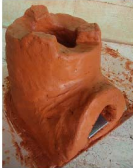
Figure 40: Example of an experimental rocket stove build together with local artisans on Totoya in 2009, made from local materials.
