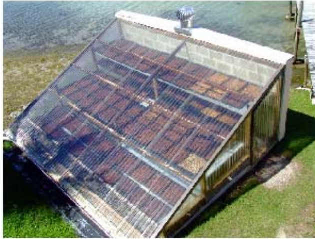
Figure 34: Small scale solar dryer on Rotuma Island, designed by John Bennett of Fiji (Photo: A. Hamm)
