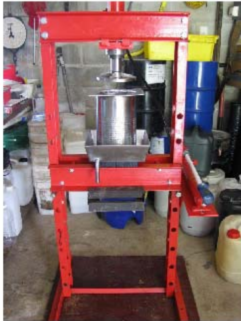
Figure 27: Hydraulic coconut oil press locally manufactured in Fiji by John Bennett (Photo courtesy of John Bennett).
